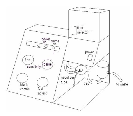
Identify the burner with its nebulizer tube for aspirating sample and waste drain tube. The trap tube between the burner and waste overflow container should be filled with water. Is it? Do not operate the burner without water in the tube. If the tube is not filled with water the propane/air mix will escape into the room.
