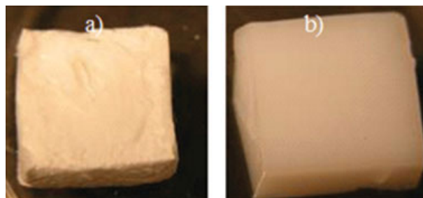
Figure 6. Image of H3 in (a) dry state and (b) swollen state. [Color figure can be viewed in the online issue, which is available at www.interscience.wiley.com .]
