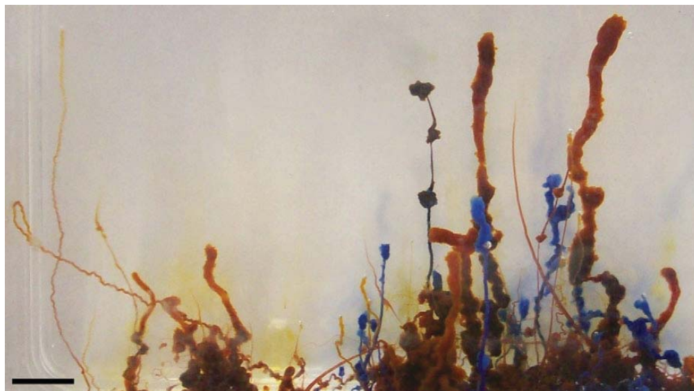
Figure 1. Tubular precipitation structures formed by seeding small particles of \text{FeCl}_3 and \text{CoCl}_2 into a 1.5 M solution of sodium silicate. Scale bar: 5 mm. (Online version in colour.)
