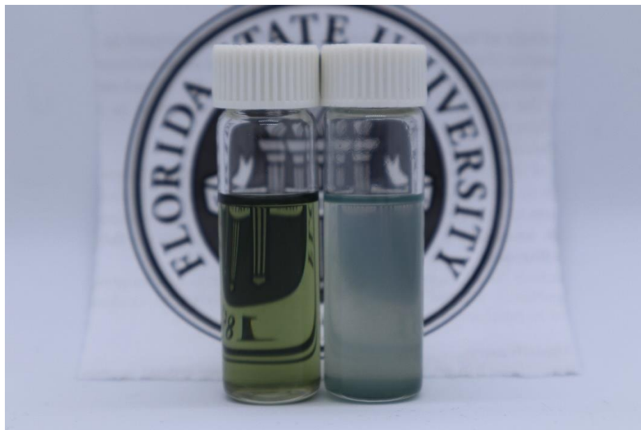
Figure 16. Picture of CTO PSNC solution in TCE (left) showing emerald color compared to a less soluble NC solution (right) demonstrating the difference in scattering between the two solutions.
