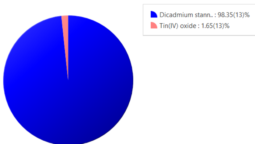
Figure 17. Whole-powder-pattern fitting (WPPF) results of CTO PSNCs using the inverse spinel structure (calc. PDF 01-080-1468) and the \text{SnO}_2 rutile structure.
