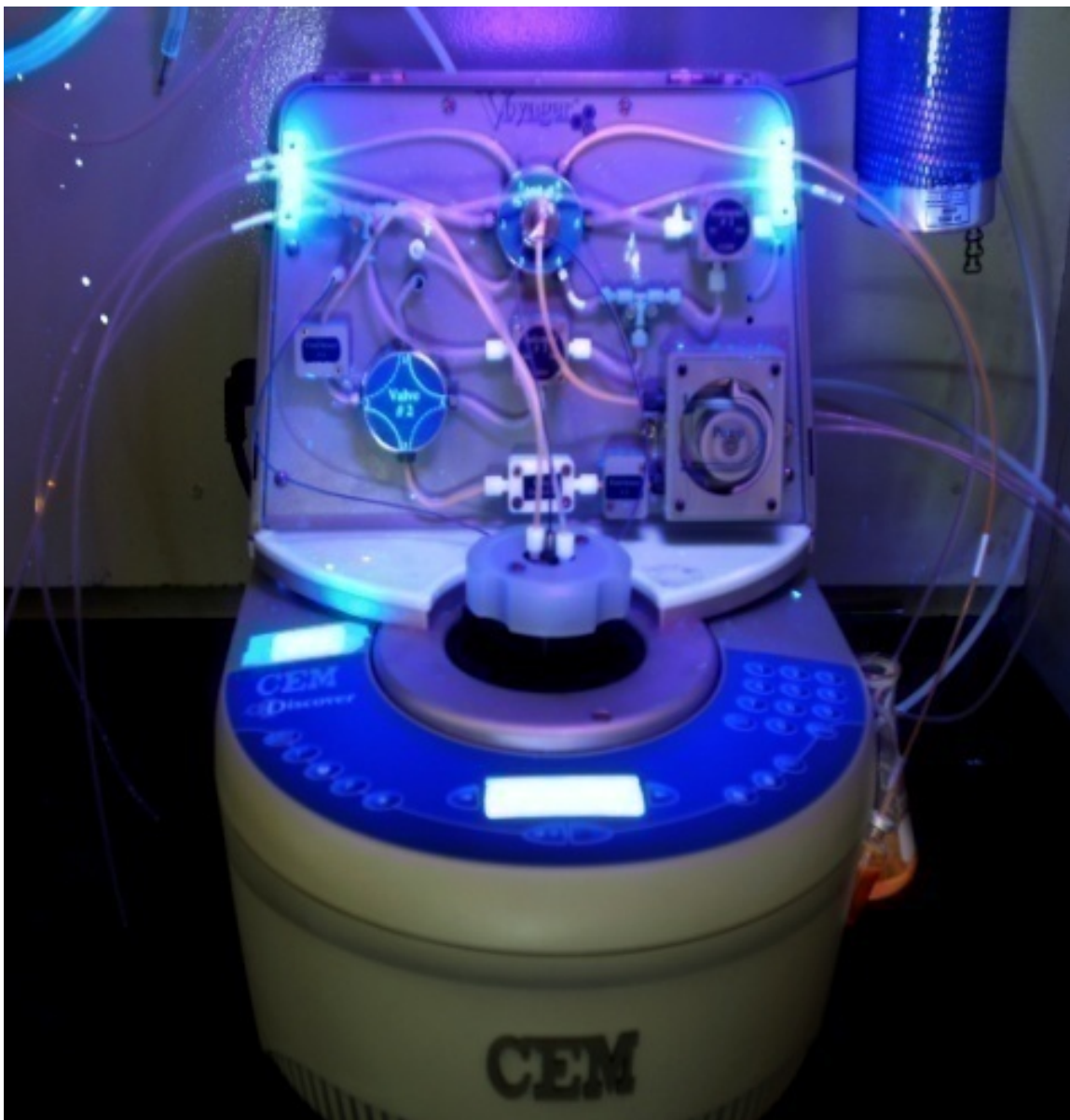
Figure 1.5. Stop-Flow Microwave Reaction
